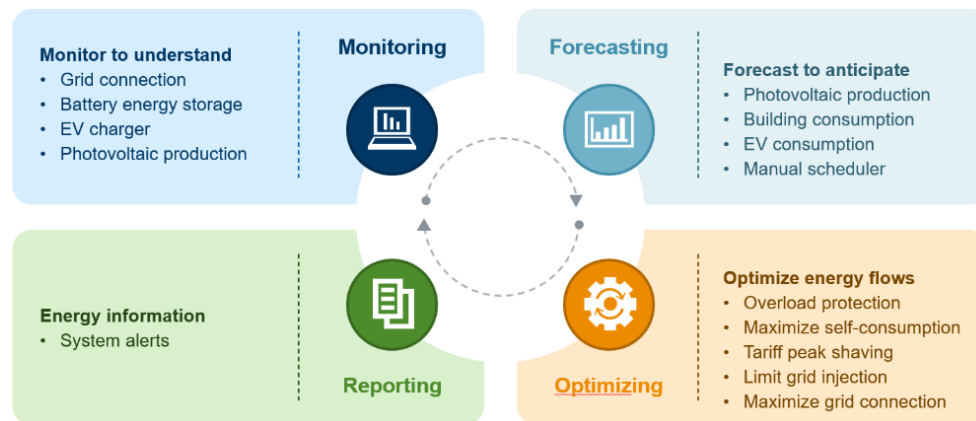
Figure 18. Energy Management System basic capabilities - EATON.
